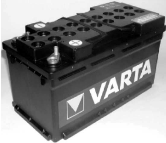
Fig. 17. The 36 V starter battery, nominal capacity: 26 Ah (C/20) AGM technology. The battery contains two rows of 18 cells. The valve openings are to be seen in the lid. Size: H 8 (EN: L5); length: 339 mm; width: 174.8 mm; height: 164.5 mm; weight: 30 kg. By courtesy of VB batteries AG.
